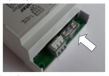
Only replace the fuse with 125mA rated, T type.
