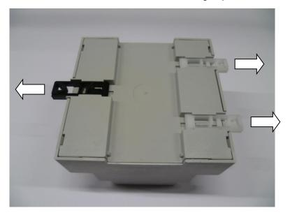
The three mounting holes can be found in the extracted clips below:
