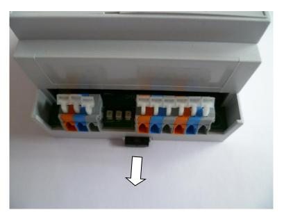
If the product is used in a situation where heavy mechanical shocks can be expected, we advise to bolt the 2 channel DMX booster directly on the surface. Extract the three mounting clips as shown here. Use bolts and nuts M4 to attach the DMX booster with the mounting clips.
