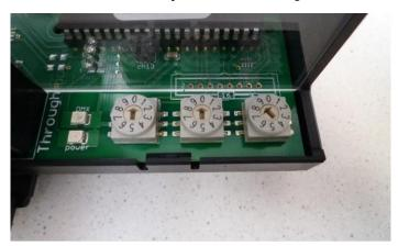
*Note*: If the card is oriented that the text on the PCB is readable, the positions of the wheels will affect following address-setting:
