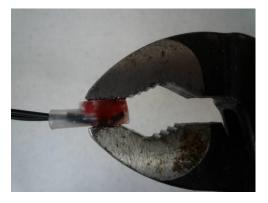
Make sure the two wires remain fully inserted in the connector.
